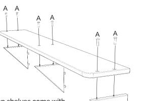
Flat-top shelves come with pre-drilled 90-degree triangles which are easily assembled with provided screws.
