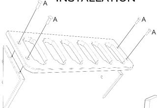
Left & right-facing Pistol Hangers are adaptable to single & double-stack mag wells. For single-stack applications, unfasten the adapter plate screws with provided hex key.
