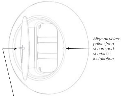
6 Locate the 9 O'clock area on clock face and press down to release from clock frame.
