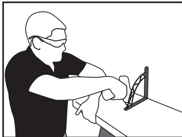
Insert screws into the TOP of the shelf with supplied 5/8" screws. See Figure 7
